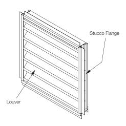
**Hinge and Subframe** Right or Left Side Option Available Stucco Flange 3/4" (19) Standard Stucco Depth
