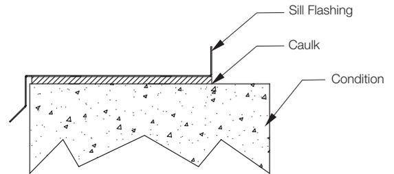
Figure 1.2 Sill Flashing Assembly
