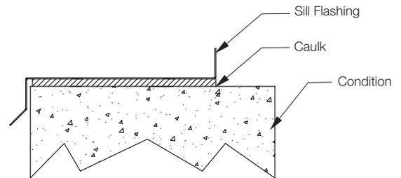
Figure 1.2 Sill Flashing Assembly
