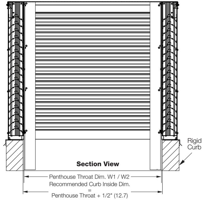
**Recommended Sizing:** (For optimum performance W1 and W2 should be  $\geq H \times 2$ )
